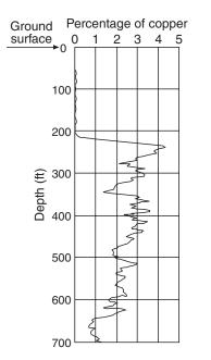
Between which depths should the bedrock be mined in order to obtain rock with the highest percentage of copper?
