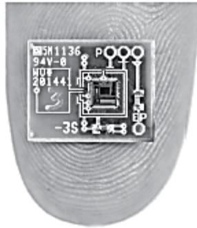
Scientists have designed a small electronic circuit (inside the two squares) that can monitor the strength of the natural battery in a guinea pig's inner ear.
