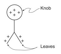
As a positively charged glass rod is brought near the knob of the electroscope, the separation of the electroscope leaves will
